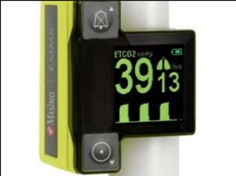
Masimo EMMA Capnograph Measures end tidal CO 2 in ICU settings
